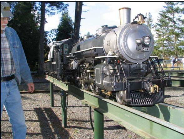
Photo Below Left: Live steam 1 1/2" scale Pacific on the service track at the Vancouver Island Model Engineers layout in Saanich.
