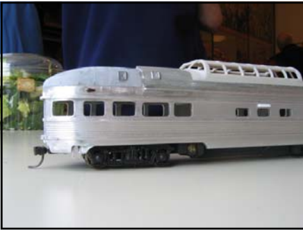
Photo Above Left: John Britt's Via Rail Park Dome Observation car is built up from an old Grandt Line extruded aluminum car. The ends were bent and new dome installed to make a proper tail end car.
