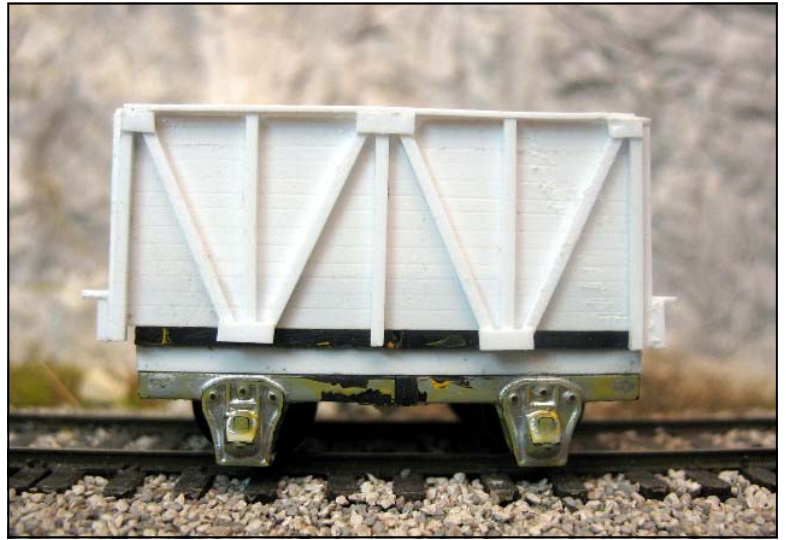
Above: All side bracing, gusset places and added frame beams are in place on the finished but unpainted side.
