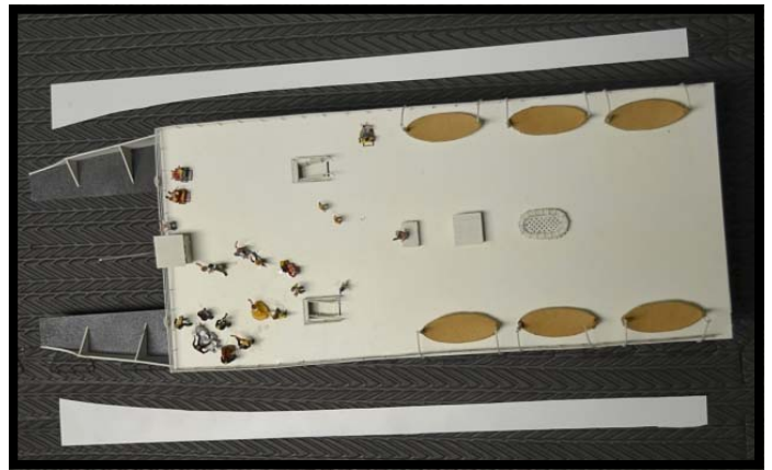
PHOTO ABOVE: In order to determine the curve required for the ferry berth 'bumper', the boat was placed on a sheet of .040 styrene and the curve of the hull traced. Once the curve was traced, the line was cut leaving about one inch of material to the land side of the curve. The two curved pieces that will provide the 'berth' curve are visible on either side of the ship.
