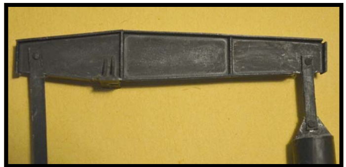
PHOTO ABOVE: The timber support column as viewed from the interior, track side. On top is the linkage that will allow the arm to move. Three 'metal' support braces are glued to a floor plate. Two additional plates will be 'welded' to the base of the arm. This arrangement is base, arm, base, arm and base. Through all five pieces a 'metal' rod is located. A 'rivet' assembly at each end of the rod assures all components remain in place.
