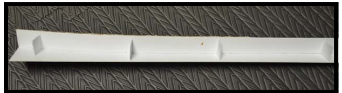
PHOTO ABOVE: A strip of styrene to be used as the wall was glued to the underside edge of the curved berth segment. The resulting L shaped assembly was braced with triangular styrene stiffeners.
