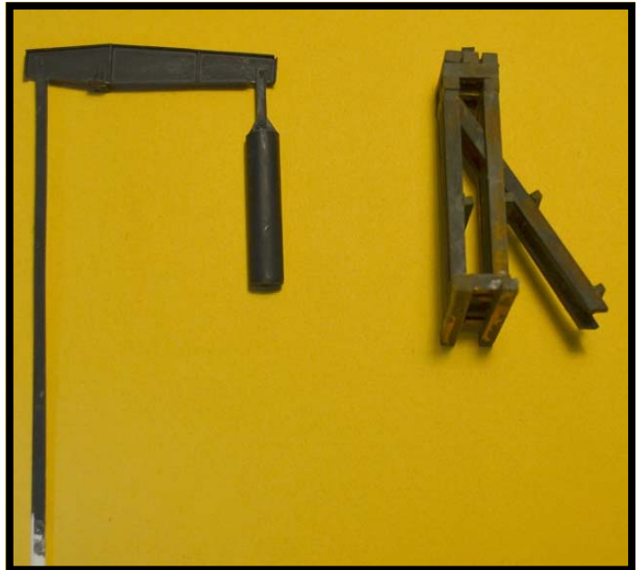
PHOTO ABOVE: The two major components of the apron assembly are illustrated above. On the left is the arm link sub assembly: attached on the right end is the steel barrel counterweight while on the opposite end is the link to the bottom of the apron. When the arm is pivoted, the link and the counterweight move in opposite directions. On the right is the timber sub assembly that supports the link, arm and counterweight sub assembly.
