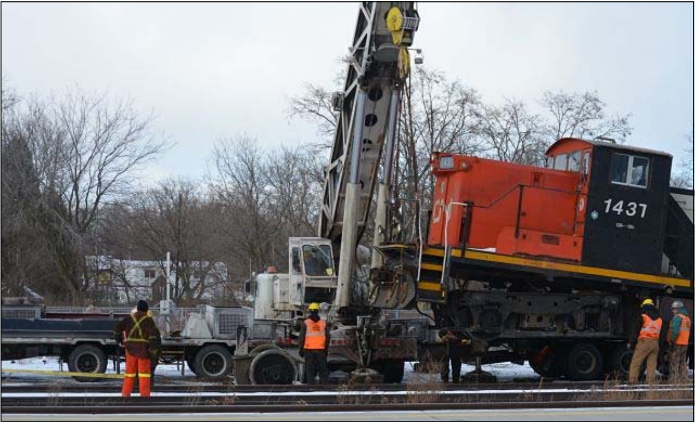
PHOTO ABOVE: The cables taught and the pulleys functioning, the cab of 1437 is raised so that the trucks release their wheel sets. The end set is pushed away and the traction set is manhandled out from underneath. Due to a difference in height between the passing track and the yard track it appears as though the wheel sets have derailed. That is not the case however.
