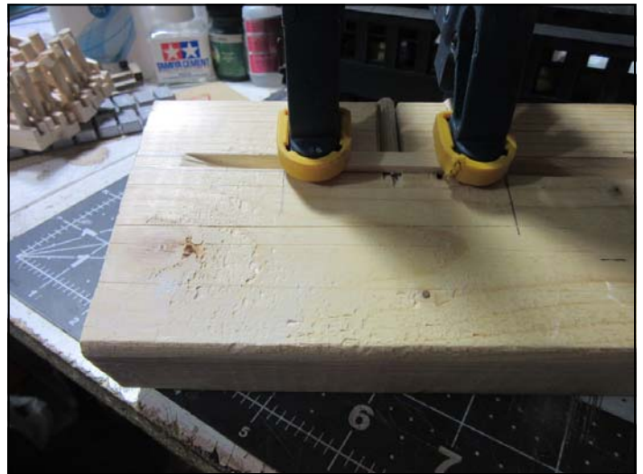
PHOTO ABOVE: The trestle sills being clamped and glued, with the radius controlled by a radius curve template.
