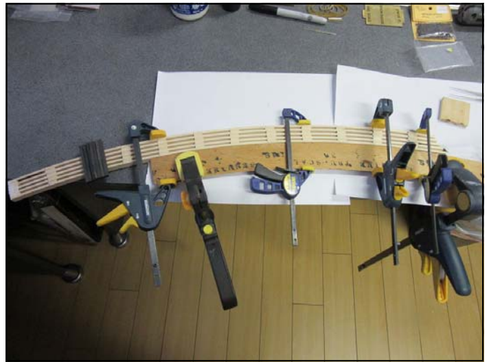
PHOTO ABOVE: the jig I made with trestle parts clamped and gluing. Note the stack of completed bents in the back left.
