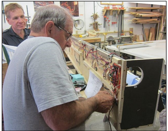
PHOTO ABOVE: Craig Dolbeer, our electronics guru, looks on as Gord Eagles makes connections on the feeder links to one of two electronic control panels in the Walkerton diorama.
