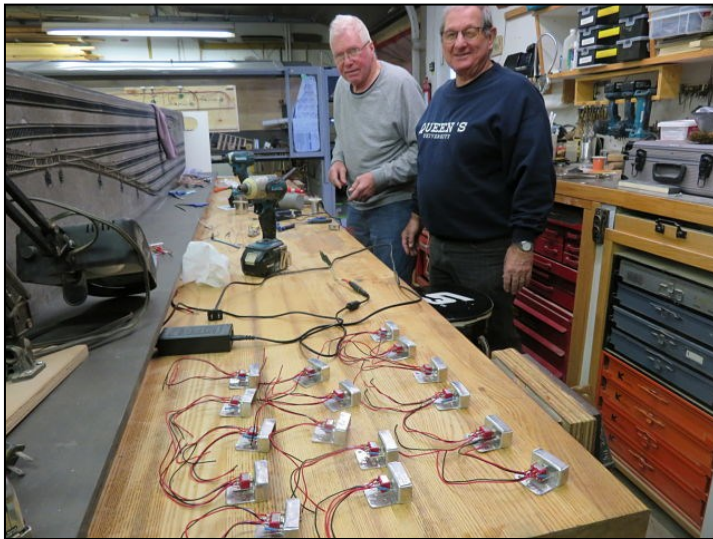
PHOTO ABOVE: Paul Maurer and Gord Eagles have just finished assembling RailCrew DPDT switches and LEDs to the custom made mounting brackets, ready to install to control the ON/OFF uncouplers.
