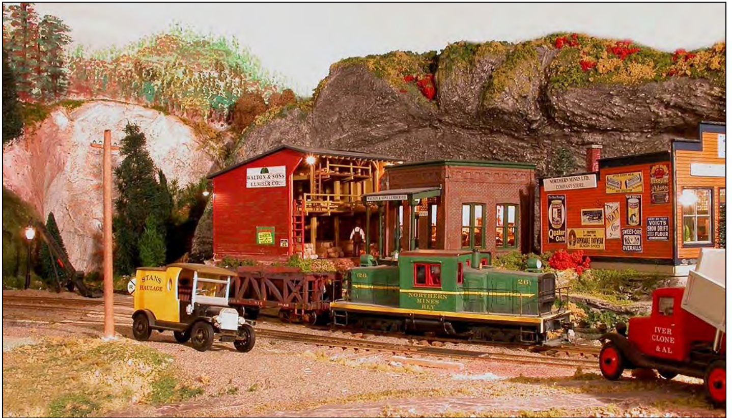
PHOTO ABOVE: One of Craig's scratchbuilt diesels is switching in the town of Northern Mines. The chassis of this diesel is an HO mechanism. Craig widened the wheel gauge and scratchbuilt the cab.
