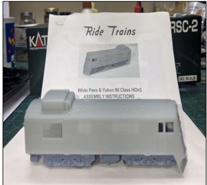
PHOTO ABOVE: The finished locomotive ready for detailing, couplers and the paint shop. As it comes the locomotive is very light. It was a challenge to find locations to install the weight. On my layout the narrow-gauge line is all level so weight was not a high priority, but I did find room for two weights.
