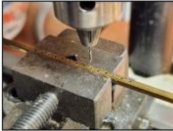
PHOTO ABOVE: Drilling out the 1/8" Square Tubing. I then cut the 1/16" brass tubing into 1/16" lengths that would fit inside the brackets.
