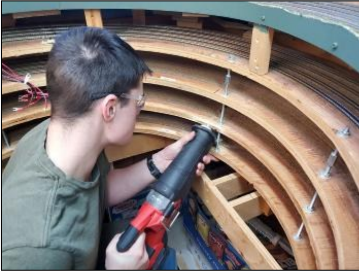
PHOTO ABOVE: My grandson Nathan starts the process by using a Sawzall to cut through the Helix. There is no road back now.
