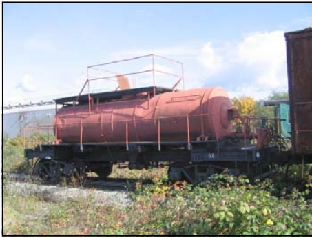
Photo Above: Ex Crown Zellerbach track watering car preceded the log train sprinkling the right of way to prevent fires caused from brake sparks. It has been restored and sits in the Port Alberni yard.
