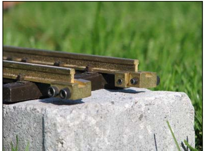
Photo Above: In this image the focus of interest are the ends of the track. George employs solid brass split jaw rail clamps as joiners for the link between sections of track. These are visible at the end of this short track. Each joiner has two Allen type screws. One screw tightens against one end of the rail, the second against the rail being joined. These joints are much stronger than a typical LGB rail joiner. These split jaw rail joiners create a positive electrical bond between each section such that George feeds the entire layout with but two feeders. He has no problem operating DCC on the layout with but these two electrical connections.
