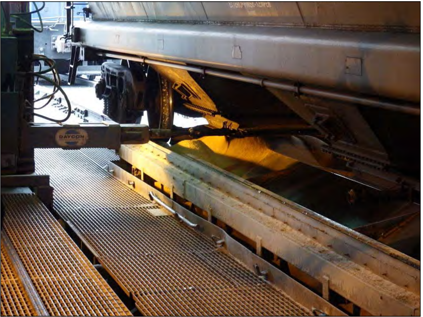
Photo Above: Walter Reid Photo: Inside the unloading building we see the Daycon machine used to open the hatches and grain flowing from the hopper.
