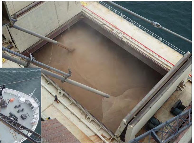
Photo Above: Walter Reid photo: As the ship is loaded, we can see that multiple nozzles are used to load the grain and even out the load in the ship's holds.
