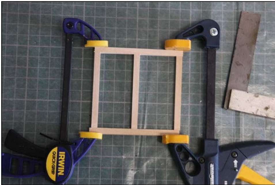
PICTURE #5 ABOVE: Clamps holding a wood framed building side while it dries. Note the background cutting board with rectangular grid lines which helps ensure squareness. The square is also useful to doublecheck all angles. Note the wax paper underneath.
