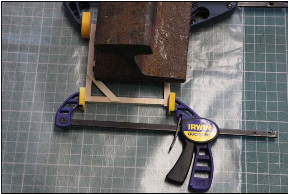
PICTURE #7 ABOVE: An alternative to the method shown in Picture #5 to glue the corner brace is to keep the frame flat on the cutting board and use a heavy weight to hold the corner bracket in place un til the glue dries. The wax paper is evident.
