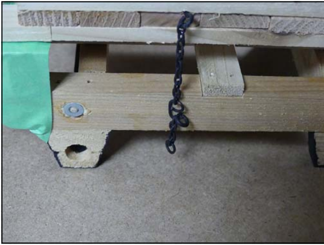
PHOTO ABOVE: Small links of chain on the car side stabilized the ore box from moving when in transit. A link was located on a horizontal J bar and the J bar twisted such that the link was unable to free itself. The green painter's tape is holding two pieces of wood together while the glue dries.
