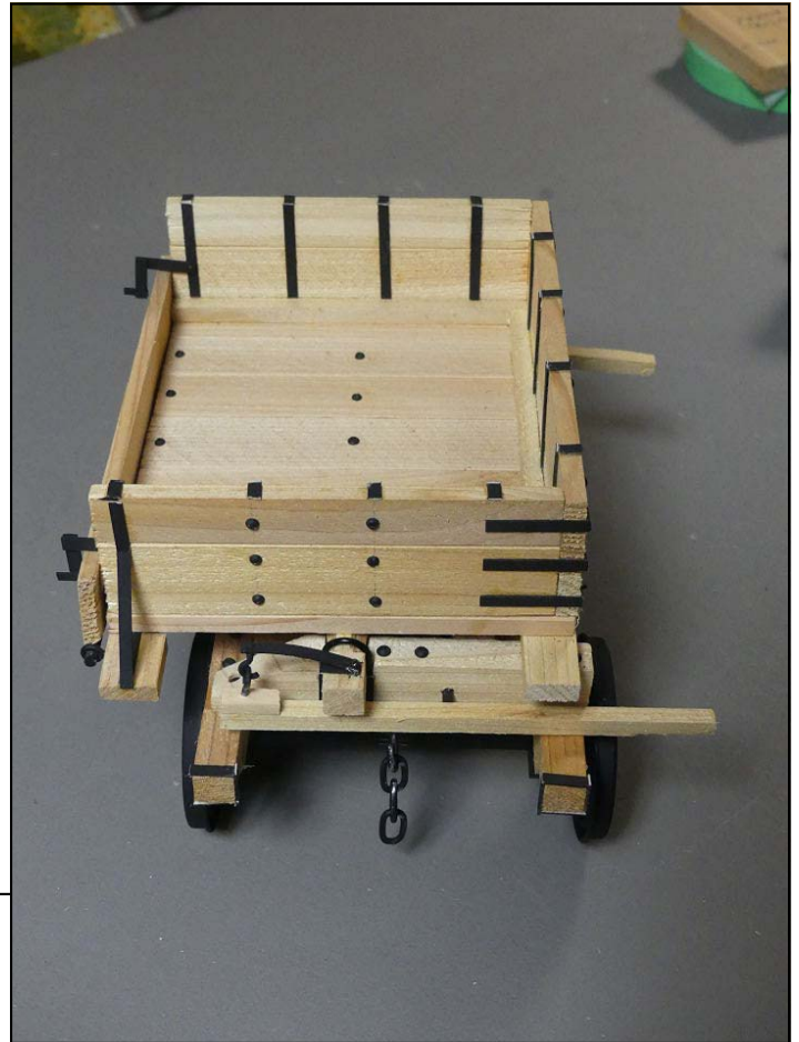
PHOTO ABOVE: This view of the end of the ore car reveals additional details. There were no brakes on these cars, save for the last one in the string of twenty-five that made up a train. The cars were coupled by three links of chain hooked onto a partially opened eye bolt, shaped like a horizontal letter J. This allowed a very tight coupling of adjacent cars but did not prevent them from buffering each other when in transit. Note the black 'iron' strapping around the end frame members. That strapping prevented the wood from splintering as the cars bumped into each other. Also visible is the spring at the end of the lifting bar. And the half circle of 'metal' that appears behind the spring allows the bottom of the box to revolve on its wooden 'axle.'
