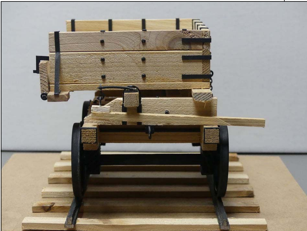
PHOTO BELOW: An end view of the completed 1867 Crossen ore car. The bar extending beyond the car on the right is the dump lever. On the opposite end of this bar is the spring. The two are mated by a hook and eye arrangement. To move the dump box into a dump position, two men, one either end, would push up on this bar and the box would tilt, allowing the ore to fall by gravity. George estimates that the two men, by exerting 115 pounds of upward thrust each, could tilt the approximate 5,000 pound load of material.
