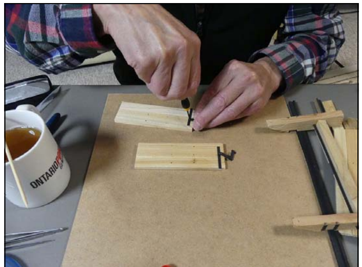
PHOTO ABOVE: Here one of the assemblers is affixing a small, very small, fastener to the wood box frame. The projection from this member will allow the box to be locked in an upright position. This securing device is 'riveted' to allow it to move. The black pieces, which appear to be metal, are in fact coloured plastic.
