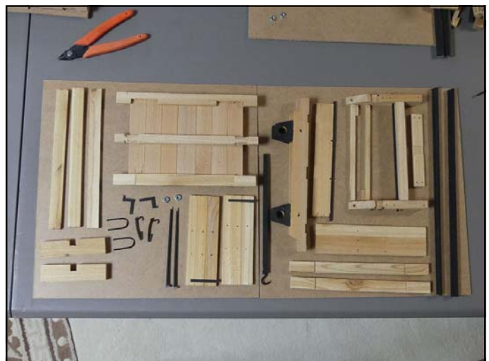
PHOTO BELOW: This image better displays most of the parts required for assembly. The bottom frame pieces have blackened 'journal' boxes through which axles will be placed. The holes in the frame are for stiffening rods, the long thin black pieces seen, and these connect the two frame pieces together with a tiny screw to secure these sides together. The bottom of the dump box frame has 3 longitudinal supports, the centre one rounded towards each end to provide the 'axle' which allows the ore body to dump. The two long strips on the left-hand side are the Masonite rails that the car will eventually rest on.
