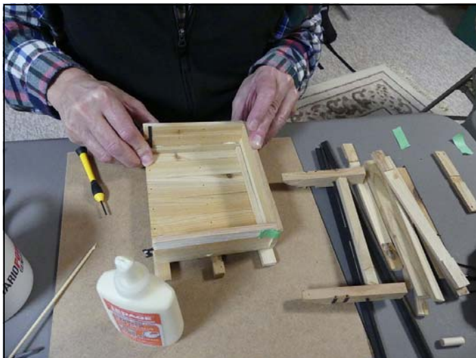
PHOTO LEFT: George recommends a quick drying yellow carpenter's glue to speed up the assembly of wooden parts. In this illustration hands and fingers are fitting the dump box sides to the bottom of the dump box. The 'U' shaped part with the bevelled ends is the part of the box frame that allows it to be tipped.
