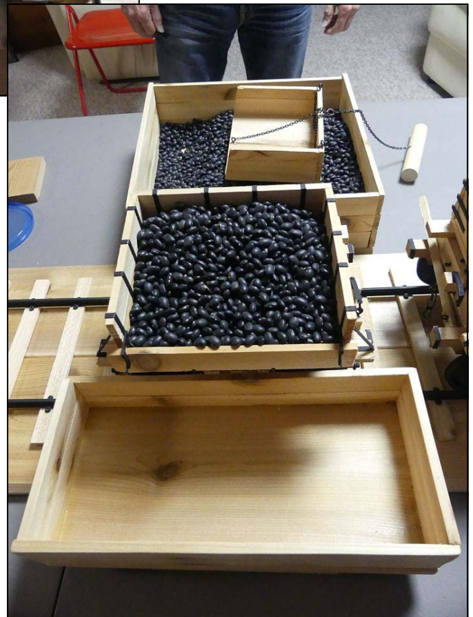
PHOTO ABOVE: In this photo modeller's fingers on the lever bars replace the arms of the men who would tip the box allowing the ore to fall out to a ship's hold or simply onto the ground, perhaps from a raised trestle to create a mound beneath. Some 'ore' has already fallen from the dump box. Voila, the proof that the two and one-half hour session of building an 1867 Crossen ore car ended successfully with an operating model. Kudos to George for his design ingenuity and his inspiring patience.
