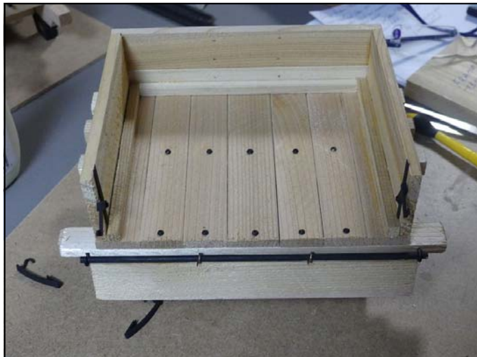
PHOTO LEFT: The box completed. Observe the rod that acts as the shank of a hinge to allow the car to side dump its contents. Note the ten miniscule black screws that represent iron bolts. Note also on the two interior box sides the moving clasp that secures the door in an upright position. The other black objects are mounted beneath the box frame and act as a leverage spring to assist in the manual dumping process.
