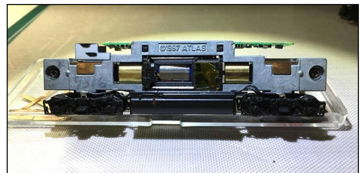
PHOTO RIGHT FIGURE 6: A decoder installation showing the space available between the frame and decoder where styrene blocks can be placed to gently force the decoder body upwards to insure a good contact.
