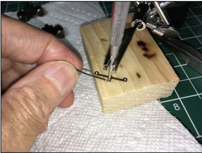
PHOTO ABOVE FIGURE 3: Soldering the 29 AWG flexible wire to the truck contact points (a "tricky bit"). The piece is held in place by impaling it onto a softwood block with a sharp -pointed tool which does not accept solder. This prevents solder from impinging on the hole which must remain open to accommodate a nub on the truck frame.
