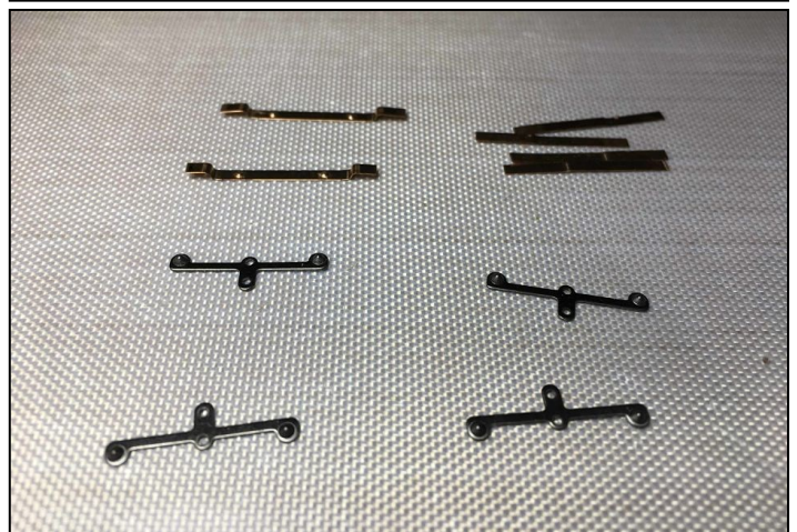
PHOTO BELOW FIGURE 2: The phosphor bronze strips after removal of 23 mm. of the contact ends (at upper right). Below are the four truck contact components.
