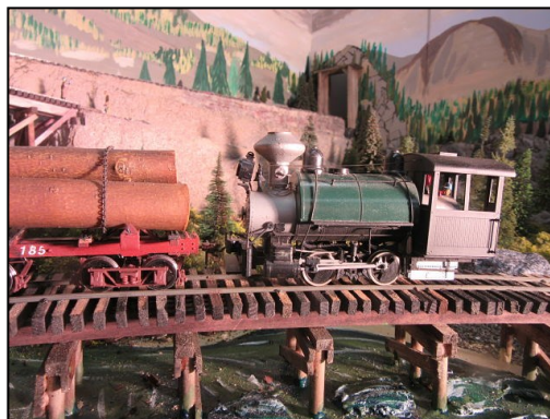
PHOTO LEFT: 0-4-0 saddle tank assembled from a Chemtron/Grandt Line kit pulls a log train in from a logging area over a trestle. These little 0-4-0s are so light and have a short wheel base. They have very poor traction and the lack of tender means there is no space for weights, decoders, keep alives etc. A Z scale decoder is installed in the cab and visible from the rear.
