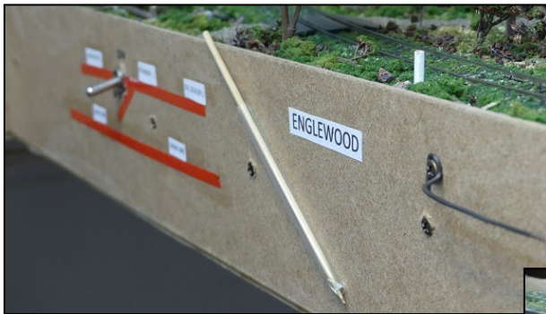
PHOTO ABOVE: An example of a track plan that appears at points about the layout. The town community is identified, a track plan is taped to the fascia, a block toggle switch controls electrical power to a particular section of track, and an uncoupling device, a pointed wooden skewer, is handily sheathed in a clear tube enclosed at one end.
