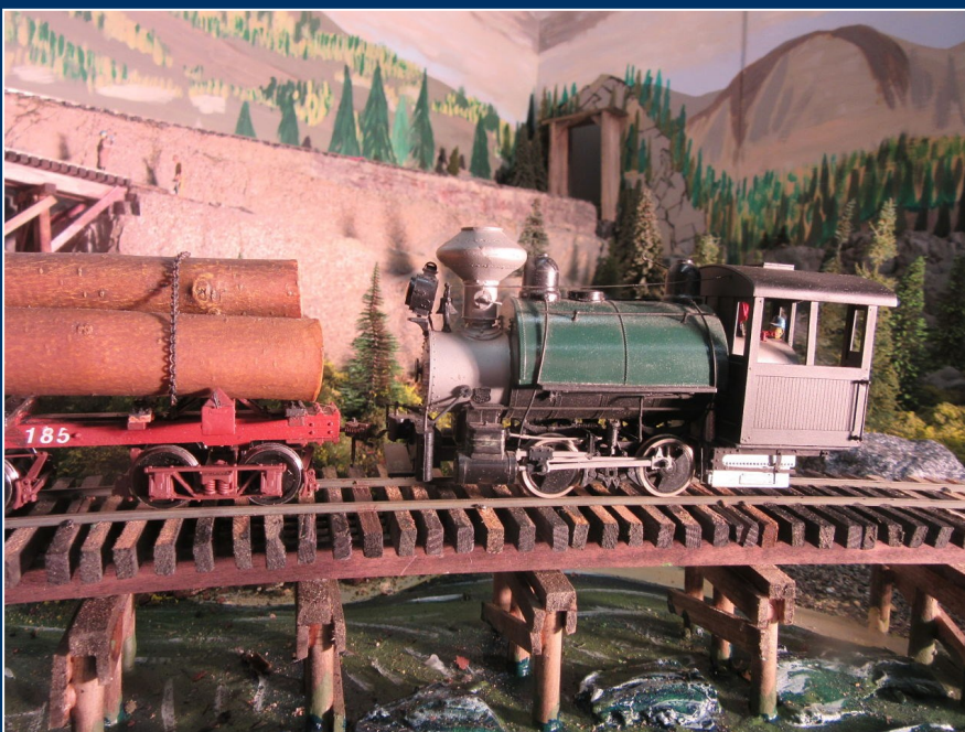
PHOTO BY GERALD HARPER: 0-4-0 saddle tank assembled from a Chemtron/Grandt Line kit pulls a log train in from a logging area over a trestle. These little 0-4-0s are so light and have a short wheel base. They have very poor traction and the lack of tender means there is no space for weights, decoders, keep alives etc. A Z scale decoder is installed in the cab and visible from the rear.
