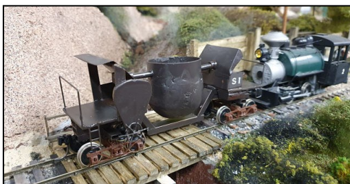
PHOTO ABOVE: Partially built 0-6-0 based on Overland 2-6-0 mechanism with scratch built body. In an 0-6-0 the boiler is long enough to fit inside the electronics needed for DCC.
