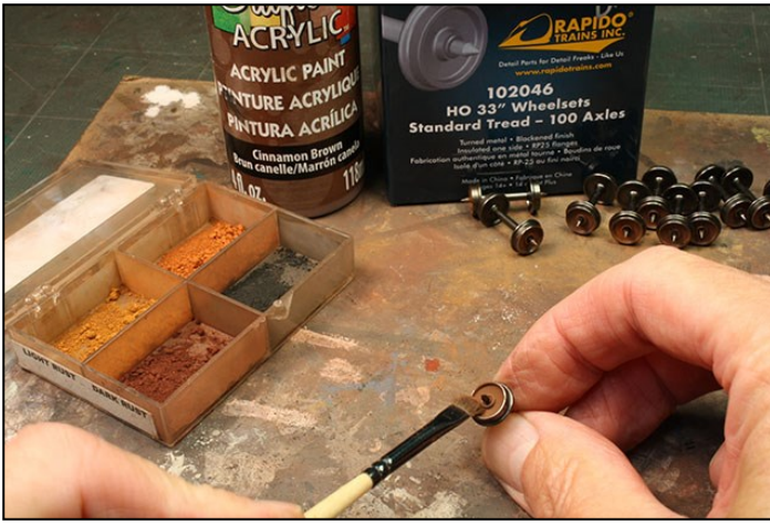
PHOTO ABOVE LEFT: Once dry the wheels receive a dusting of Bragdon powders.
