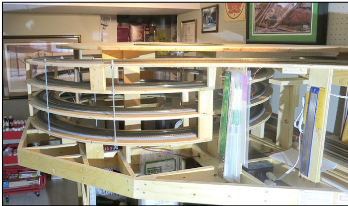
PHOTO ABOVE LEFT: A view of the helix. You can see the threaded rods used to support the levels.
