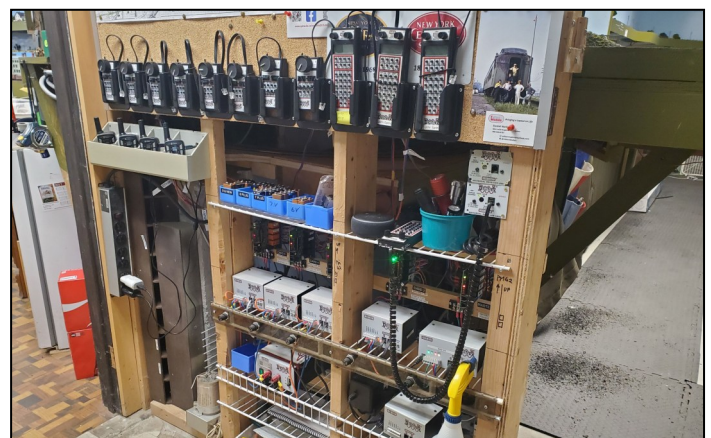
PHOTO BELOW: The Digitrax Command Station and Booster units to control the layout along with operators throttles are all centrally located.
