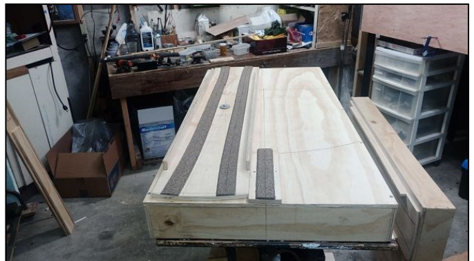
PHOTO BELOW: Showing the leg socket. A 2x2 leg slides in and is held in place with a keeper pin, allowing the turntable to be picked up and moved during setup. A temporary piece of 2X2 has been inserted to test fit everything.
