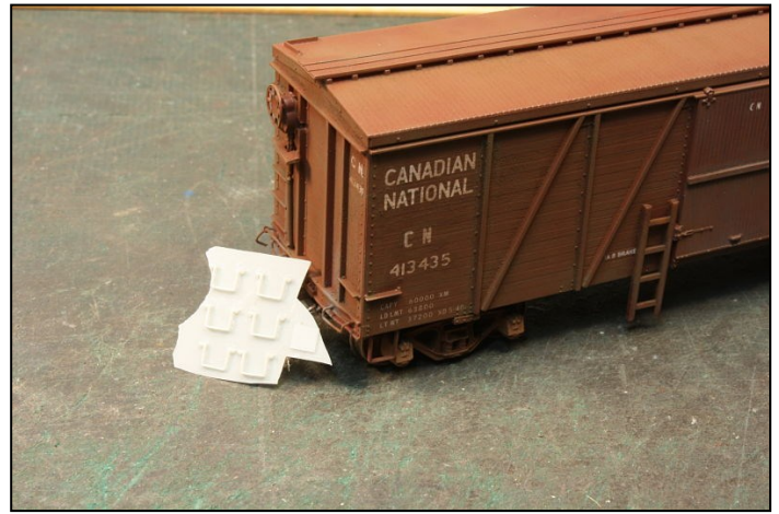
PHOTO ABOVE: Once completed I realized that I did not add the end stirrups by the ladder. F&C leftovers are used.
