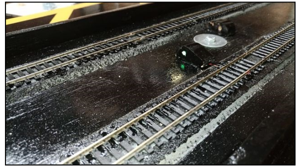
PHOTO ABOVE: The lock mechanism can be seen. This was formed from a section of chromed piano hinge. The approach track pieces are two inches long, the turntable pieces are one inch long. I drilled two extra holes in each piece for screws. The bolt is 4 inches long and bent into an L shape with a 1 inch handle. Track feeders are short pieces of flat brass bar stock, soldered to the rail and pinched under the lock mechanism.
