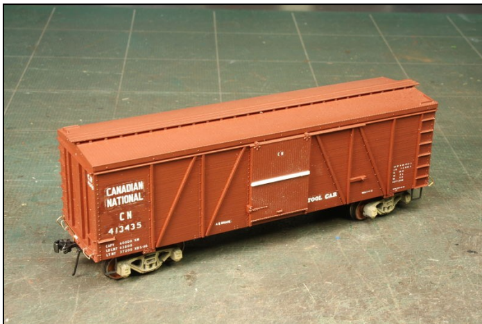
PHOTO ABOVE: The decals and details are applied to the model and are ready for painting. A gloss coat and flat finish will be also applied to the car hiding the decal seams.
