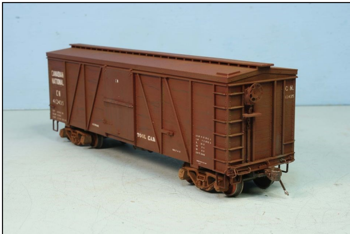
PHOTO ABOVE: The decals and details are applied to the model and are ready for painting. A gloss coat and flat finish will be also applied to the car hiding the decal seams.
