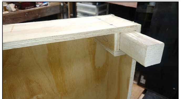
PHOTO BELOW: Showing the leg socket. A 2x2 leg slides in and is held in place with a keeper pin, allowing the turntable to be picked up and moved during setup. A temporary piece of 2X2 has been inserted to test fit everything.
