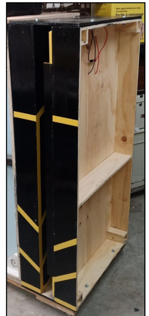
PHOTO ABOVE: The shoulder bolt pivot point is just visible between the tracks. This provides the pivot. There are two fender washers, identical to the one visible under the pivot bolt, between the turntable and the base to provide as smooth bearing surface.
