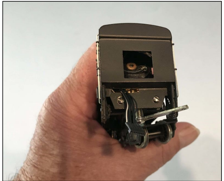
PHOTO 5: Slot cut in cab rear wall, TCS micro connector passed through the slot.
