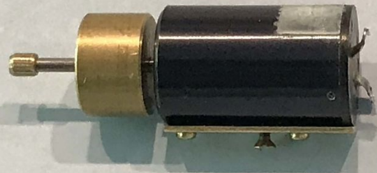
PHOTO 2: NWSL can motor on brass mounting plate with flywheel & bushing attached.
