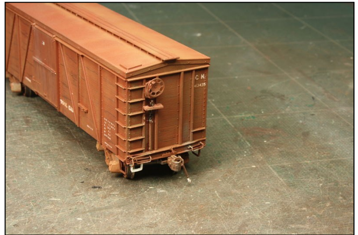
PHOTO ABOVE: The end stirrups and brake wheel chain are applied and ready for touch up painting.
