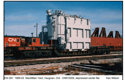
KW-391 1989-03 MacMillan Yard, Vaughan, Ont. CN672005, depressed center flat Ken Wilson
