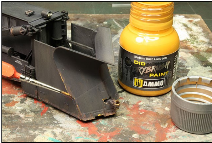
PHOTO ABOVE LEFT: MIG Drybrush paint is being applied to highlight some areas of the model that would have found chipped away base coating. George Dutka photo.
