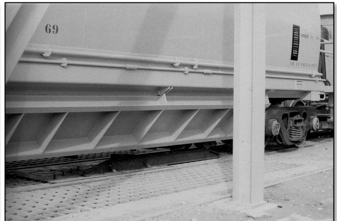
PHOTO ABOVE RIGHT: Bottom gate closed.
