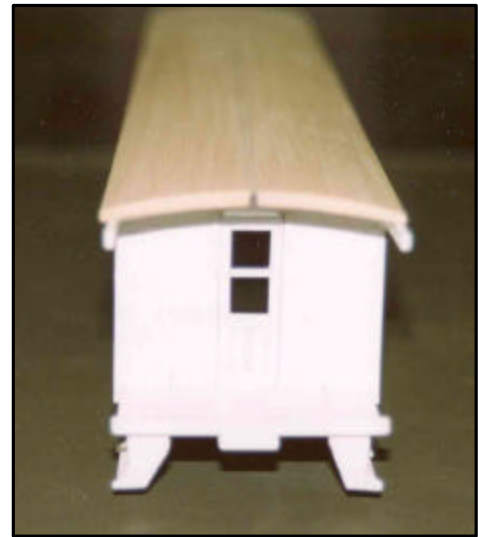
PHOTO #4: A block of hard maple was sawn and planed to the appropriate size for the roof. The final shapes were drawn on the block. A notch was cut around the roof so that the finished roof sat down into the sides and end walls 1/16". This flange is necessary to keep the side walls straight and also to remove the roof portion for painting and installing the seats and window glass
