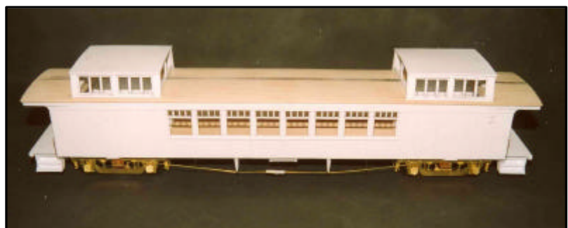
PHOTO #8: The roof cupola and windows were cut and assembled from 0.20" styrene
