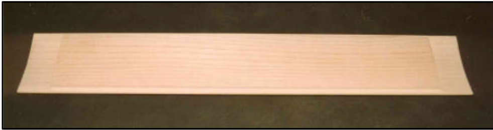
PHOTO #4: A block of hard maple was sawn and planed to the appropriate size for the roof. The final shapes were drawn on the block. A notch was cut around the roof so that the finished roof sat down into the sides and end walls 1/16". This flange is necessary to keep the side walls straight and also to remove the roof portion for painting and installing the seats and window glass
