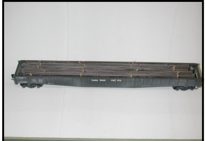
Photo 8: CPR mill gondola loaded with rods. Rods made from steel wire. Model by Ray Hoadley.
