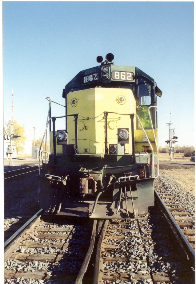
Photo 4: Oops! That wasn't supposed to happen. A Dakota, Missouri Valley & Western GP38 split a switch at Flaxton, North Dakota
