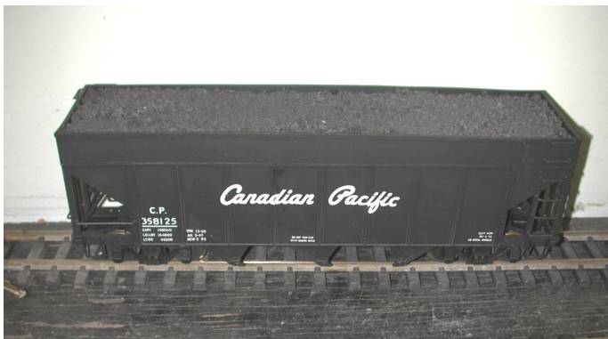
Ray Hoadleys G Scale model of CPR 358125 with 3 ft extensions for carrying coke.
