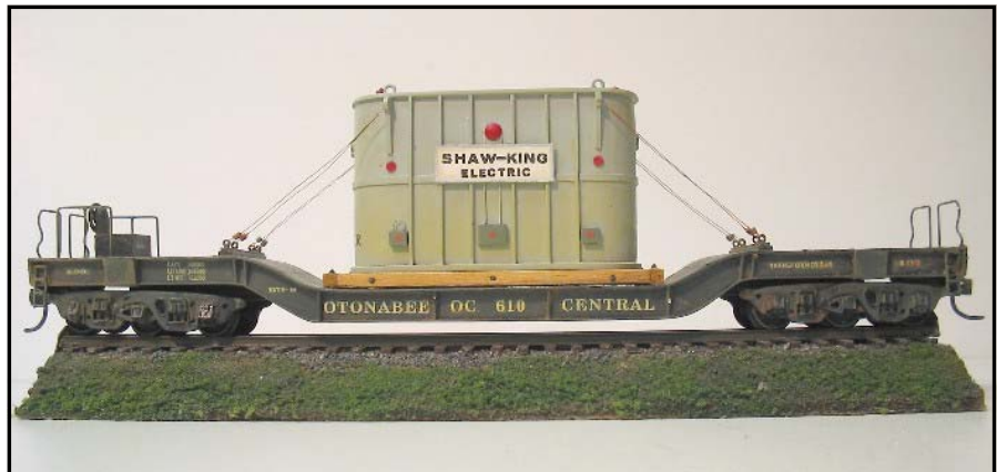
Photo 7 Left and Photo 8 Below: Alex McLeod became so involved in the contest he actually made 5 depressed center flat cars for his Otonabee Central Railway. The car contains a hidden Athearn passenger car weight which provides enhanced rail adhesion for the car. The car frame is constructed from .005 styrene. A sewing pounce tool was used to create the rivet detail. The transformer load is fabricated from shaped balsa wood and styrene. The tie down rings are tabs from KD coupler pockets.
