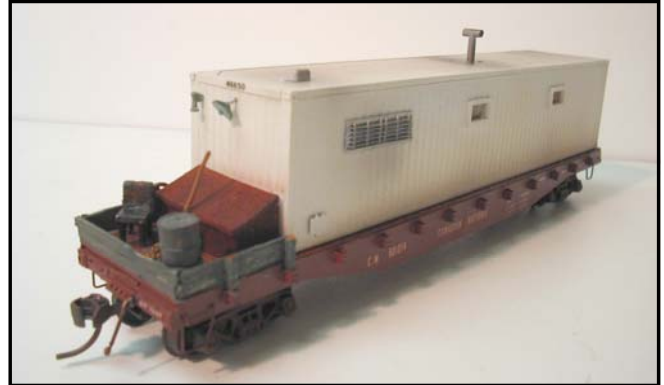
Photo 10 Right: Ron's flat car has BB's hidden in the centre channel which are used to provide weight in the car. The load is a container which has been heavily modified as seen in the photo to represent a contemporary maintenance of way car.
