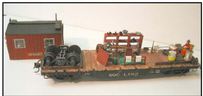
Photo 4 Below Left and Photo 5 Below Right: Cold Creek railway flat car #45 along with Snow Plow #1 originated from the fertile mind and deft hands of Dave Mehew. Fabricated by DAVBILT Locomotive and Car Works, the length of the flat car is 22 feet in On30. Styrene sheet and structural shapes are the basic building materials for the car, the cabin, and the wings. The wings are moveable and the cabin and wings are both removable so the car serves as a flat car. The stone weight was cut from a paving stone.
