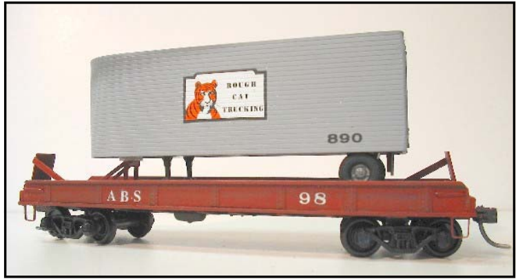
Photo 6 Above: Conrad Hill placed two HO flat cars in the contest which threw the judges into a tizzy, as there were only “nine” contestants. Judging by elimination would not work. Conrad had always wanted a piggyback car so he began with an inexpensive gondola. The sides were cut down and the car shortened. The ends were cut but the poling pockets were retained. An Athearn truck body was the basis for the piggyback load. The round front was formed from styrene sheet.
