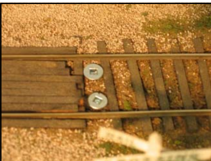
Photo 4 Above: Steel screws to hold rare earth magnets in place
