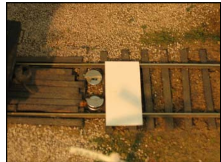
Photo 6 Above : .020 styrene height gauge
