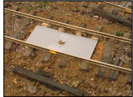
Photo 2: Kadee steel backer plate installed with a #3 screw.
