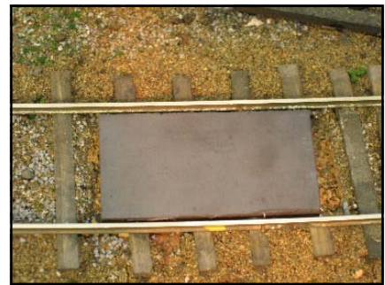
Photo 3: The large Kadee slab is unsightly unless a level crossing is available to disguise it.
