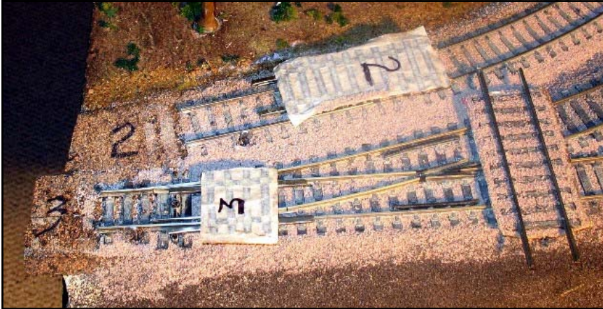
Above: Track splices created a challenge. The three needed track splices were cut and rail joiners, able to slide towards the centre of each track splice, were added. These track segments fit on top of the profiled cork roadbed. Masking tape wider than the ties was attached along the bottom of the Peco Flex Track as a base for ballast. The splice locations were numbered and the corresponding number was also placed on the bottom of the masking tape. Ballast was glued in place and when inserted on the modules, the splice is minimally visible.
