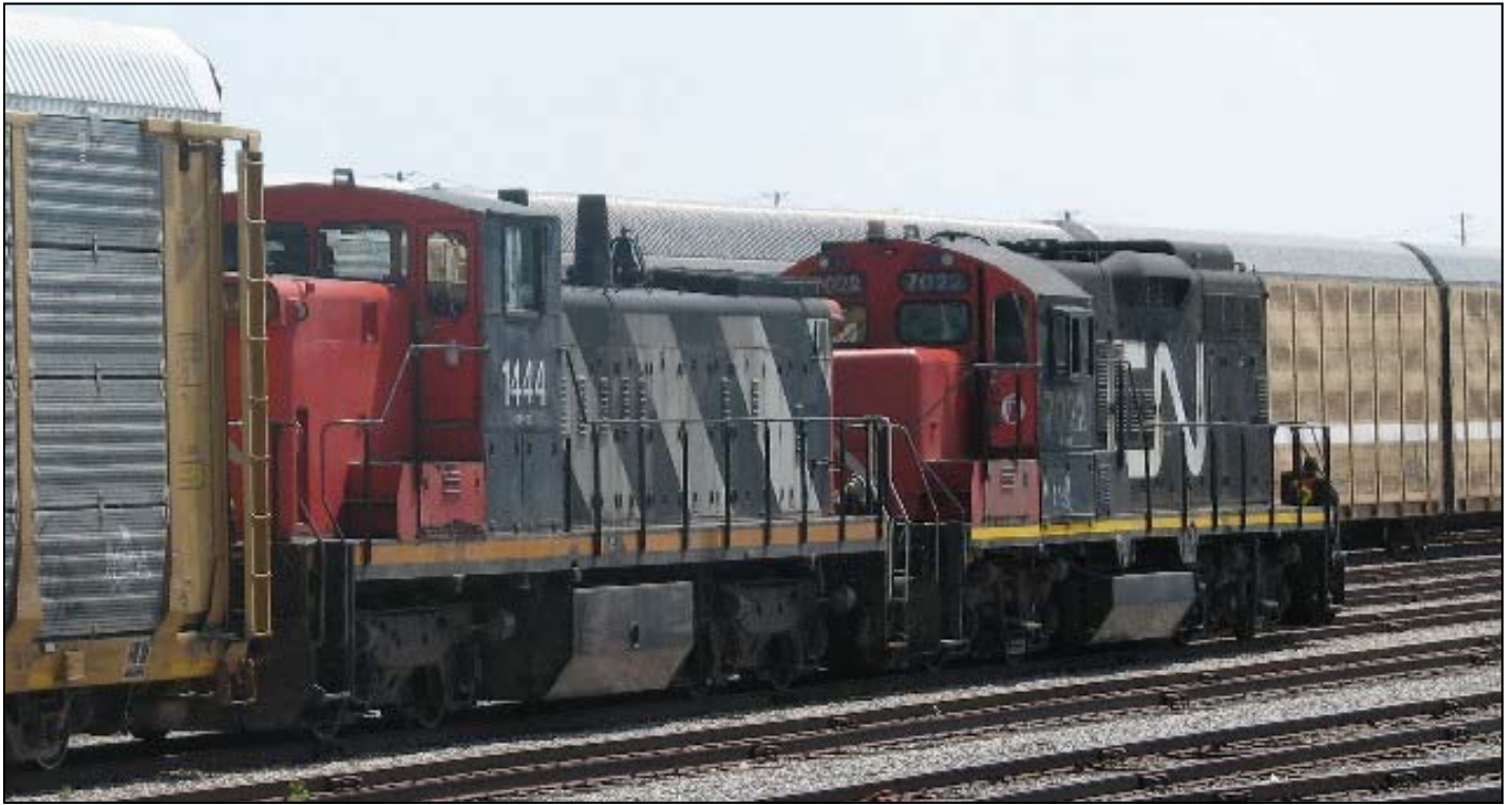
A uniquely Canadian locomotive, there were 101 GMD1's built in two classes between August 1958 and April 1960. 101 of these engines were built, however only 31 on CN's roster today. Engine #1444 is seen below working at the Ford Motor Plant in Oakville on July 19, 2011. #1444 was rebuilt in February 1998. The engine had originally been #1614, built with A1A-A1A trucks. It was the first of the 1600 series to be rebuilt and received 4 wheel B-B trucks as part of the rebuild.
