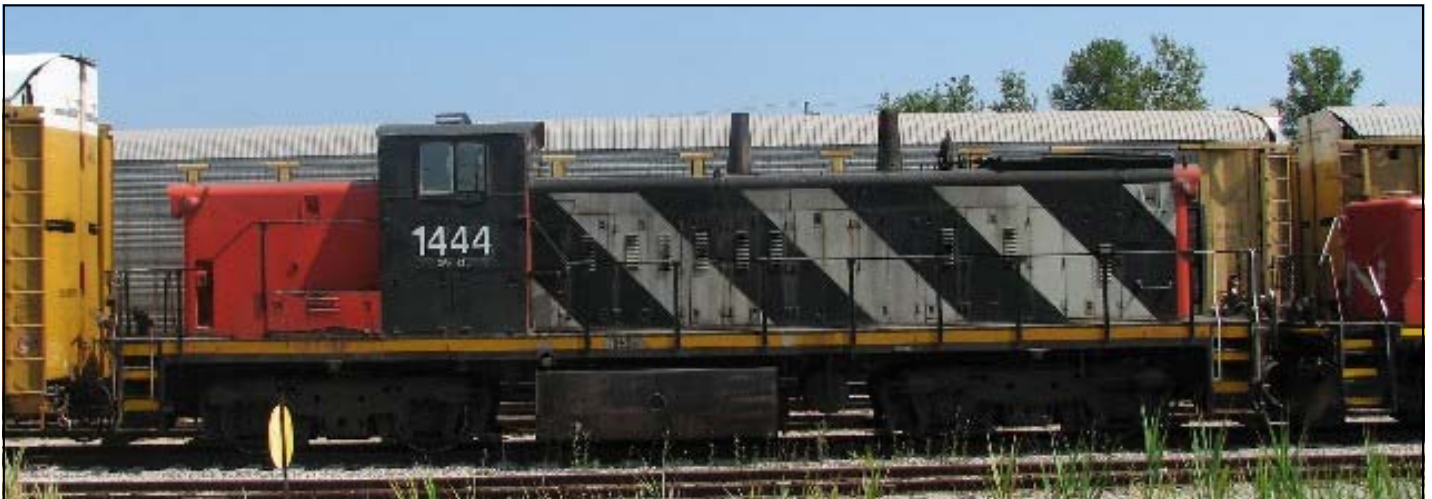
A uniquely Canadian locomotive, there were 101 GMD1's built in two classes between August 1958 and April 1960. 101 of these engines were built, however only 31 on CN's roster today. Engine #1444 is seen below working at the Ford Motor Plant in Oakville on July 19, 2011. #1444 was rebuilt in February 1998. The engine had originally been #1614, built with A1A-A1A trucks. It was the first of the 1600 series to be rebuilt and received 4 wheel B-B trucks as part of the rebuild.
