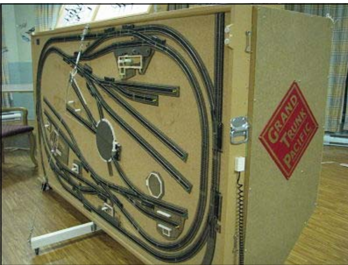
Photo Above: The layout in its vertical storage position. The sheet is stabilized by two wire supports attached to the outrigger on wheels which stabilizes all for the trip to storage.
