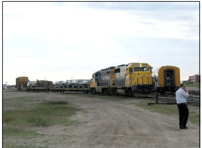
Photo Bottom Right: Crewman on the ground gives instructions over the radio to the road crew of the Polar Bear Express who are bringing the head end and automobile flatcars from the loading area to couple onto the front of the passenger cars which can be seen to the right of the train. The fully assembled train will then be brought forward to the station for passenger loading.
