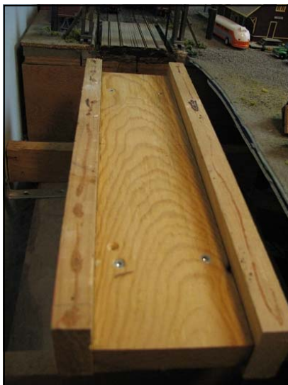
Photo Left: This U shaped structure, firmly attached to the layout, holds a two track car deck, an integral part of the ferry model, and the only part not made from styrene. It has been in place for more than a decade.
