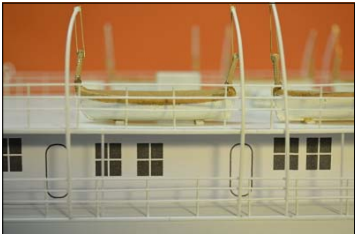
Photos Below: The Promenade Deck windows and doors were created with a computer program, printed on ordinary paper, and affixed to the walls with an aerosol glue. This image provides a view of the posts and railings that were added to each deck.
