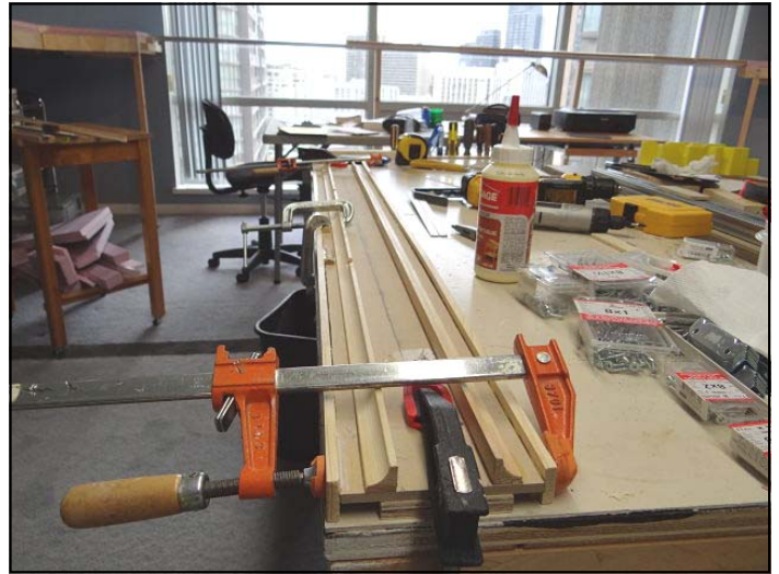
PHOTO 15 ABOVE: The wooden structure which will support the rails on the bridge (inverted). The steel girder will fit into the central channel (black clamp)
