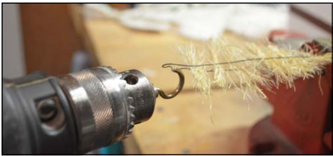
Image 7 This sequence involves inserting the stem of an elongated cup hook into the chuck of an electric drill. Place the cup hook into the looped end of the florist's wire. Slowly power the drill so that the wire is twisted onto itself and secures the hemp fibres along the 'trunk' of the tree.
