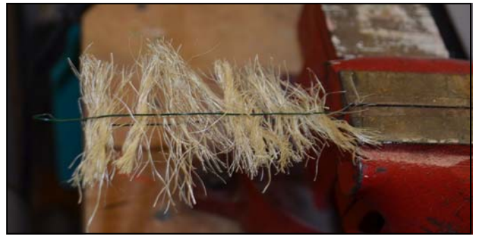
Image 6 Next take the assembled wire and hemp to a vise and clamp the loose ends of the wire into the jaws of the vice.
