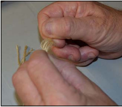
Image 3 Next step, twist the hemp fibres apart between thumbs so that the spread apart.
