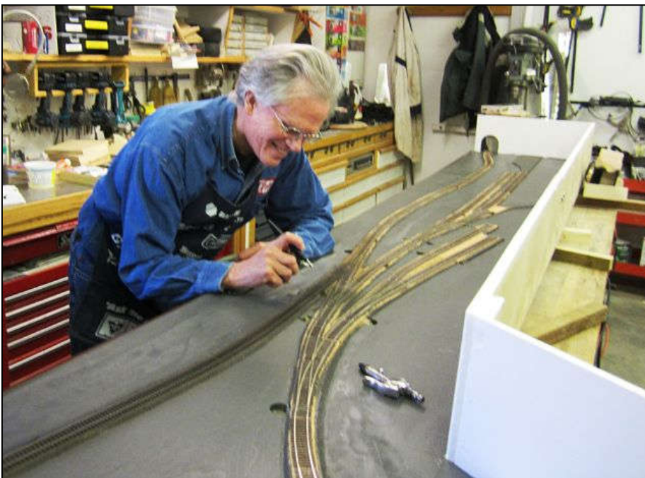
PHOTO RIGHT: Sometimes modifications to the frames are required to accommodate track curves. All track was tested using 80 foot Rapido passenger cars and Athearn passenger cars with 6 wheel trucks.
