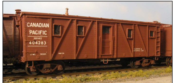
PHOTO ABOVE & PHOTO BELOW: The CP boarding cars have had windows, a stack for the stove that supplies heat on cooler evenings and a side door once the freight car door is removed added to them.
