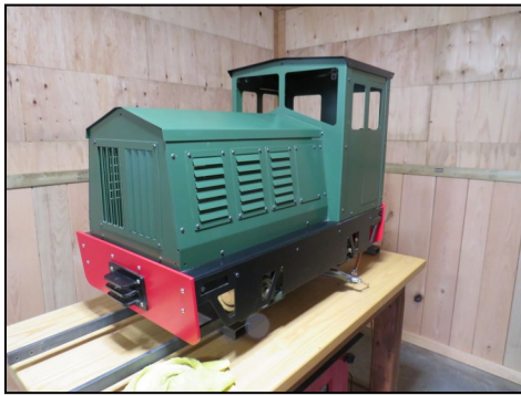
TOP LEFT: Hunslet Switcher Power: 24volt battery, Manufacturer: Phoenix Engine Works, UK, Owner: John Park
