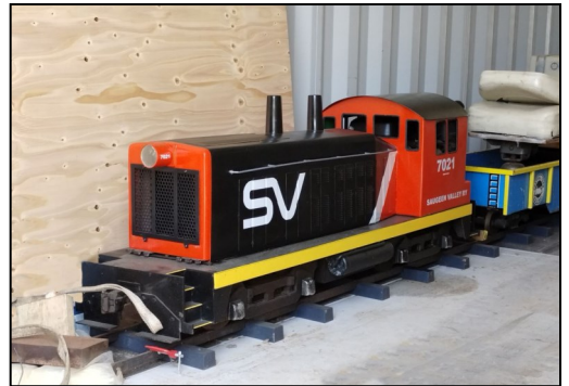
BOTTOM RIGHT: GMD SW1200 Power: 4HP Gas Engine/Hydraulic Drive Manufacturer: Morris Railroad Supply, US Owner: Doug Martin
