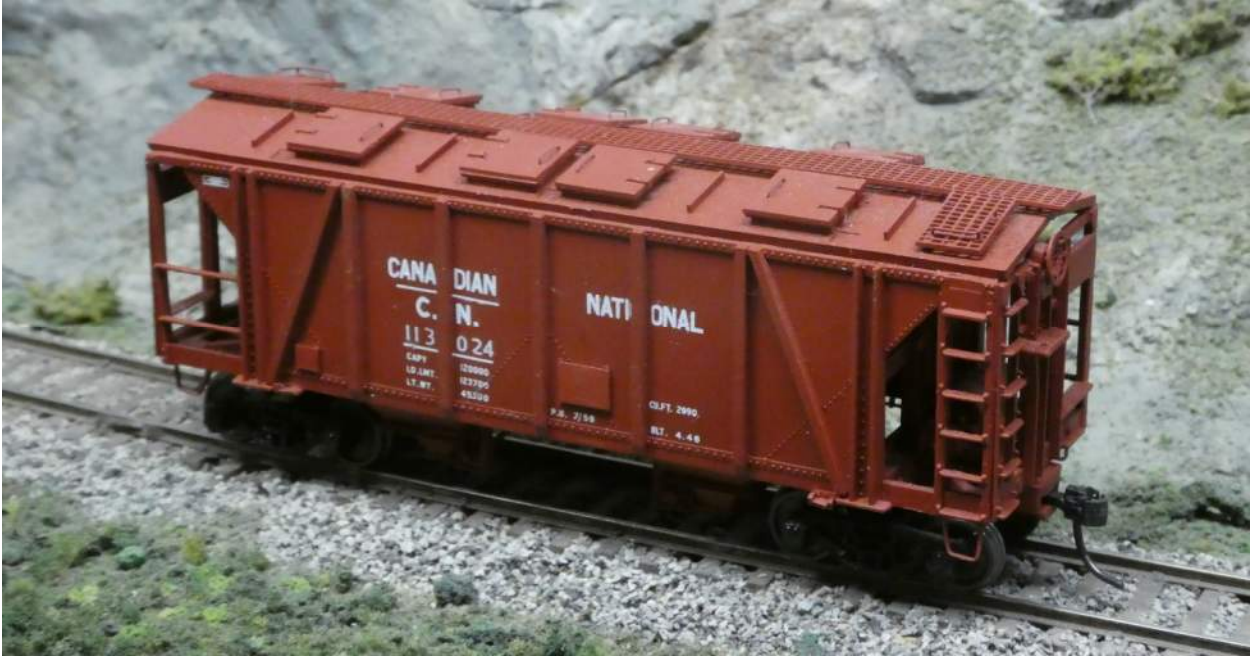
P – 278 is an E&B Valley 1948 ACF 2-bay hopper modified to CN with applied rivets
